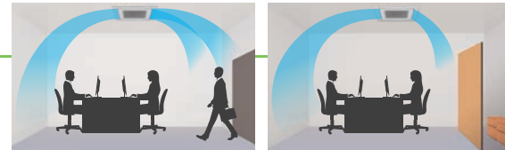
Airflows avoid blowing cool air directly at the occupants in the room, providing more comfortable air conditioning. Provides efficient air conditioning based on the room layout.
