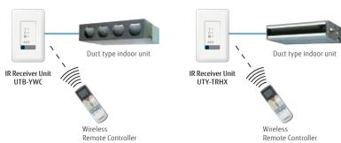
Duct type\* indoor units can be controlled with Wireless Remote Controller
